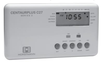
The Horstmann CentaurPlus C27 two channel programmer gives independent control over hot water and heating with up to 3 ON/OFF settings for each day of the week. It also has a 1 hour manual boost button for the hot water and an advance button for the central heating.
